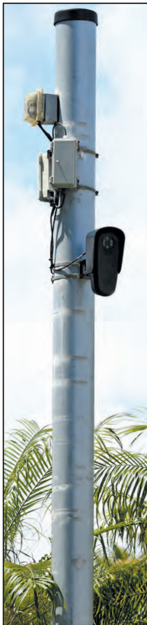
Technology advances have led local police departments to invest in systems that improve results in fighting crime. LEFT and TOP: License plate reader cameras mounted on major streets are linked to real-time systems that alert police to information such as arrest warrants and expired vehicle tags. Ocean Ridge Police Officer Aaron Choban keeps track in his squad car. ABOVE: Boca Raton uses a robotic dog as part of its bomb squad. Photos by Jerry Lower/The Coastal Star and provided
